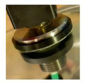
Nautilus Marine Service GmbH has done intensive inhouse pressure tests to 700 bar as well as long-term leak tests at low pressure to assure the integrity of the through-wall connector system.
